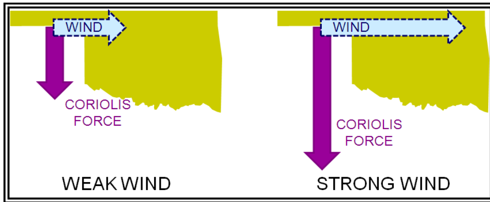
Figure 10-5. Coriolis Force Magnitude Variations with Wind Speed
