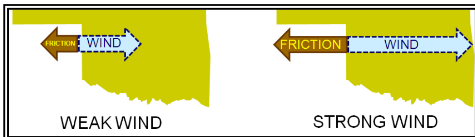
Figure 10-7. Friction Force Magnitude Variations with Wind Speed
